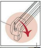
ADJUST THE BELT: if the belt slips on the machine when walking). Start the treadmill and increase the speed. If the strap slips, use a 6mm wrench, turn the bolts on both sides 1/4 clockwise. Repeat this procedure until the strap is tight.
