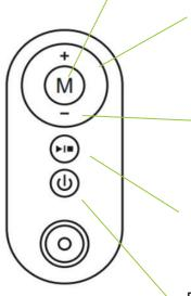
**Speed +** (Speed Plus key): After starting the treadmill, the speed increases. After pressing the treadmill once, the adjustment range is 0.1km/H. When the treadmill is pressed continuously for more than 1 second, it continues to increase.
