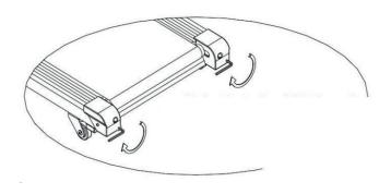
TIGHTEN THE DRIVE BELT: If the drive belt becomes loose after using it for a period of time, you should:
