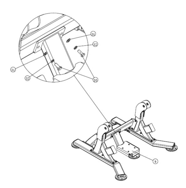
Attach Elbow Pad Support (#10) to Central Connection Frame (#8) and Right Bottom Frame (#2) using:
