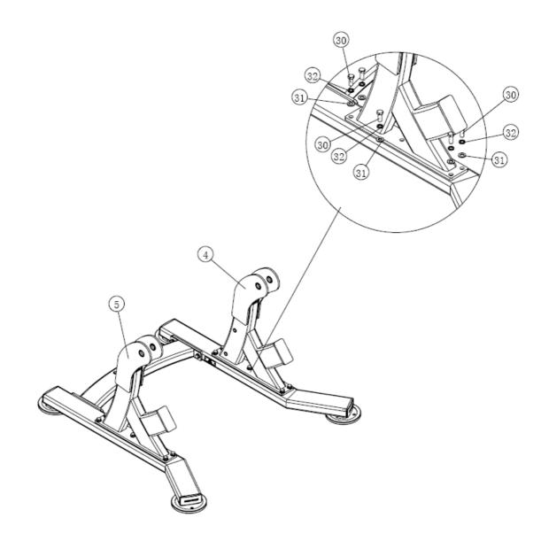
Attach Right Bottom Frame (#2) and Left Bottom Frame (#3) to Central Connection Frame (#8) using:
