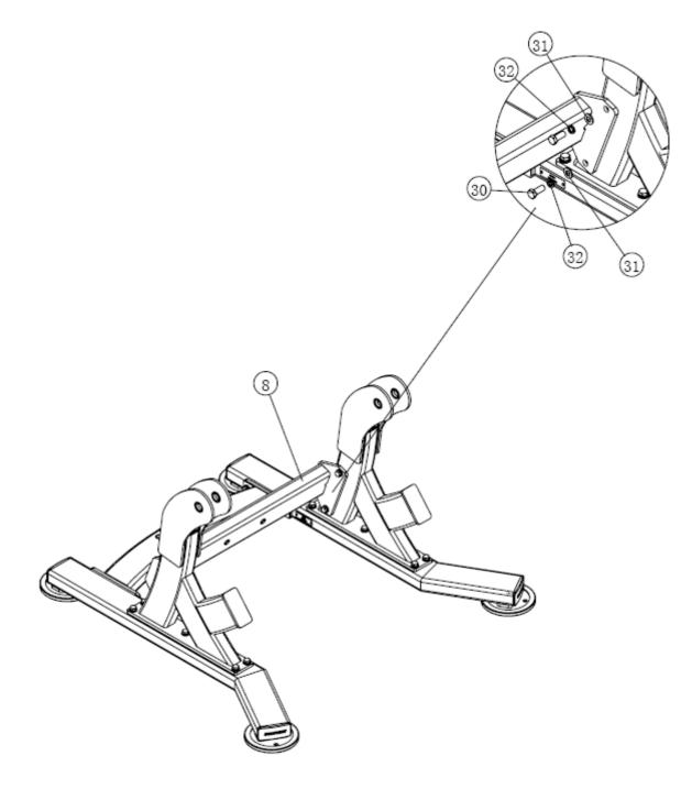
Attach Pedal Fixing Frame (#9) to Central Connection Frame (#8) using:
