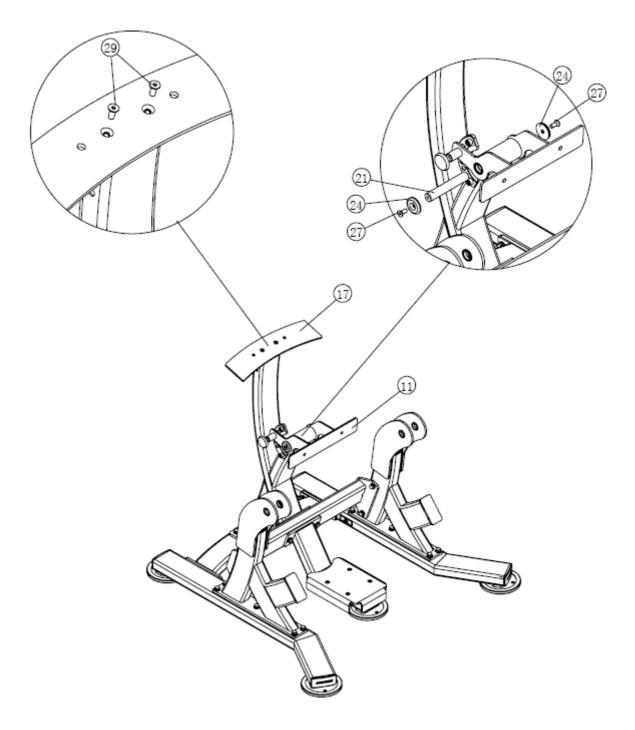
1. Attach Leg Pad (#18) to Foot Pad Support (#11)
