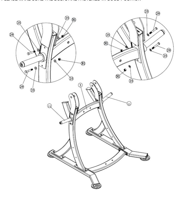
1. Attach Vertical Frame Assembly (#2) to Bottom Connection Frame (#1) using:
