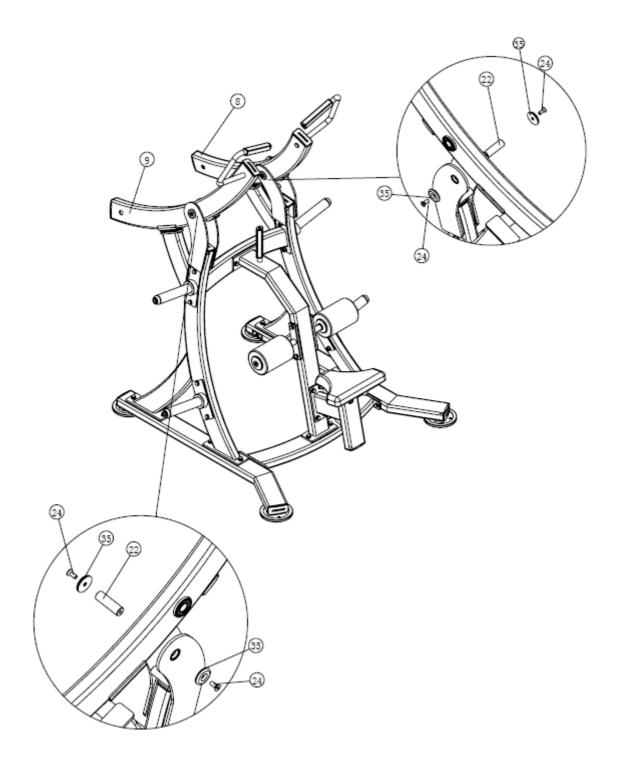
1. Attach Longer Barbell Plate Rack (#13) to Right Arm Frame (#8) using:
