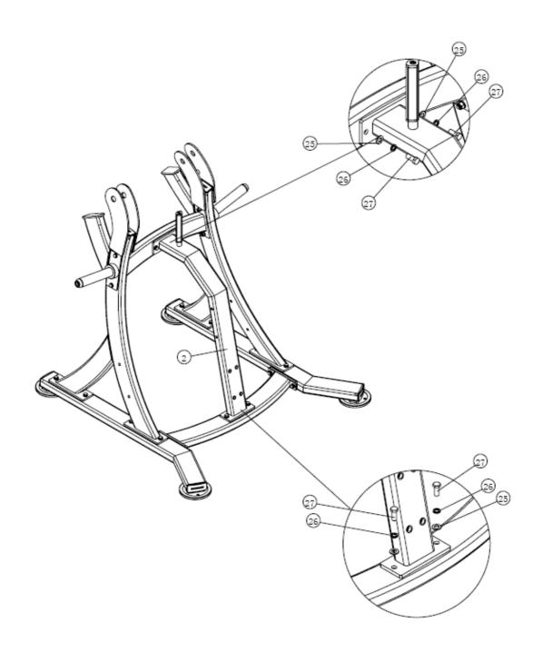
1. Attach Seat Support Frame (#12) to Vertical Frame Assembly (#2).
