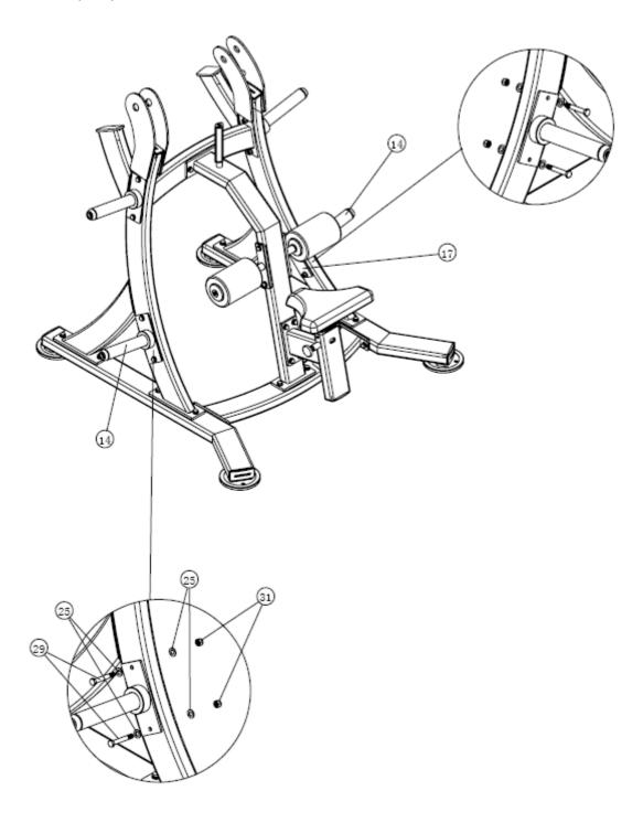
1. Attach Right Arm Frame (#8), Bearing Rotating Axle (#22) to Right Vertical frame (#6) using:
